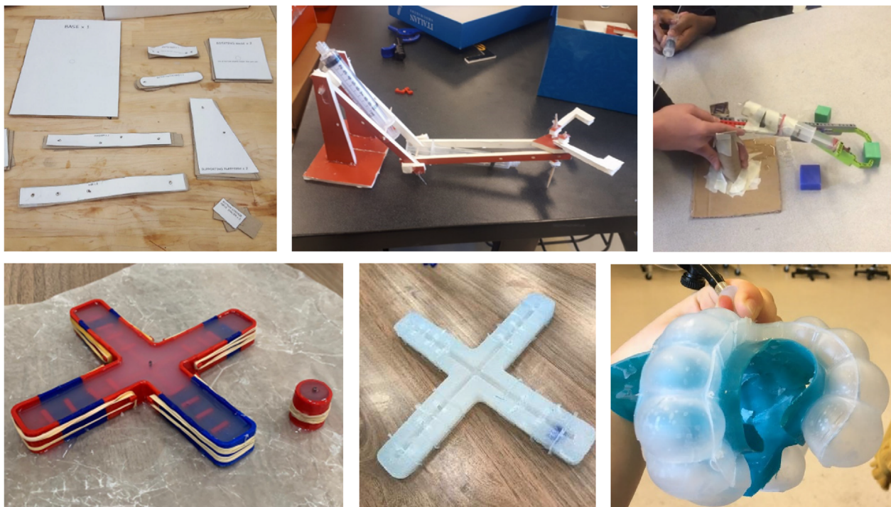
FIGURE 1 Student fabrication examples from the rigid (top row) and soft (bottom row) robotics lessons. Cutout rigid components (top left) and example rigid robots (top middle and right). Molding silicone (bottom left), cured and demolded material (bottom middle), and inflated soft robot (bottom right) [Color figure can be viewed at wileyonlinelibrary.com ]
